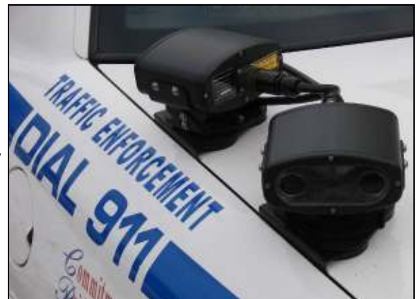
The newly acquired mobile license plate reader checks registrations of passing cars against databases for a variety of offenses, sounding an alarm for the officers to take notice of a wanted plate.
